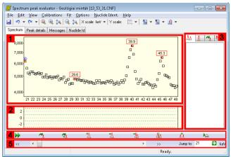
Main window of spectrum peak evaluator appears now. The center of the window is occupied by the **spectrum window [1]** and the **residual window [2]**. The residual window displays the difference between the measured counts and the fitted peak curves. A **region list panel [3]** is placed on the right, while a **fit fine tuning toolbar [4]** and a **navigating toolbar [5]** is at the bottom. List of fitted peaks is displayed under the Peak details tab.
